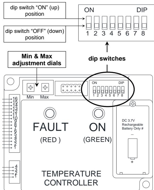
13. If adjustment is required, using a phillips head screw driver turn the "MAX" dial anti-clockwise to increase the maximum burner gas pressure or clockwise to reduce the maximum burner gas pressure, whilst reading the gas pressure on the manometer.
