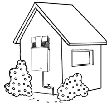
This water heater must be installed vertically upright with the water and gas connections on the underside, pointing toward the ground. The back of the water heater can be either against a wall or supported by a frame.
